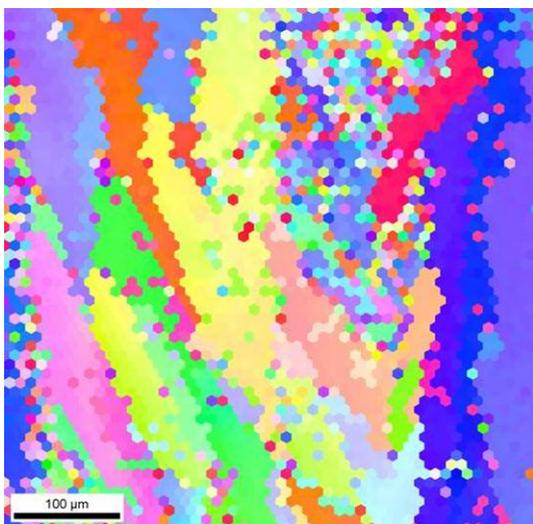
**Figure 11:** EBSD map of a 500 nm thick ESPC layer deposited at 47 nm/min and annealed at 650°C for 1.5 h.
