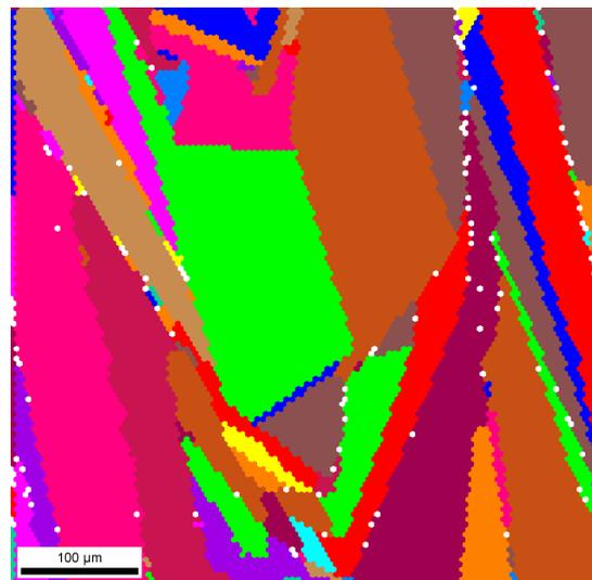
**Figure 4:** EBSD map of a diode laser crystallized seed layer on glass.
