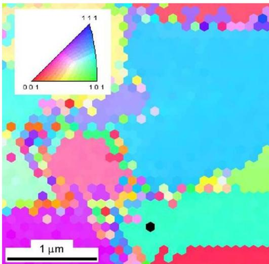
**Figure 1:** EBSD map of a 1.1  $\mu\text{m}$  thick a-Si layer on glass deposited at 100 nm/min and SPC crystallized by annealing at 600°C for 11 h.
