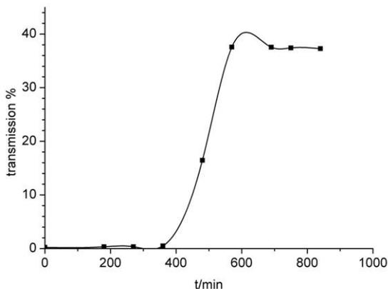
**Figure 2:** Evolution of transmission of an a-Si layer on glass deposited at 100 nm/min during annealing at 600°C
