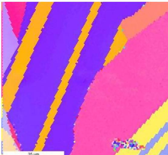
**Figure 6:** EBSD map of a layer system of a 500 nm thick ESPC layer annealed for 5.5 h at 600°C on top of a laser crystallized seed.
