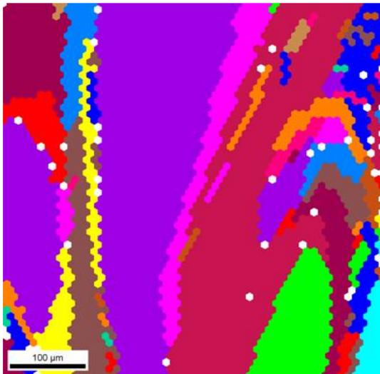
**Figure 9:** EBSD map of a 1 μm thick ESPC layer deposited at a rate of 180 nm/min and crystallized by annealing at 600°C for 12 h.
