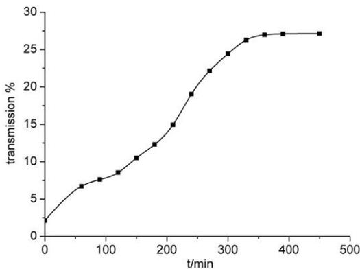
**Figure 5:** Evolution of transmission of a 500 nm thick a-Si layer deposited at 90 nm/min on a seed layer during annealing at 600°C.
