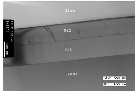
**Figure 7:** TEM cross section image of a layer system consisting of ESPC layer (Si2) on seed (Si1) after annealing for only 7 h at 600°C.
