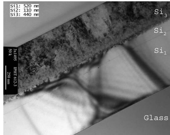
**Figure 12:** TEM cross section image of an ESPC layer on seed (Si1) annealed at 650°C for 6 h showing an epitaxially crystallized layer (Si2) and a fine grained layer (Si3).
