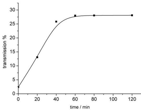
**Figure 10:** Evolution of transmission of a 500 nm thick a-Si film on crystalline seed during annealing at 650°C.
