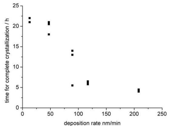
**Figure 8:** Time needed for complete ESPC of a 500 nm thick a-Si layer on top of a seed at an annealing temperature of 600°C.
