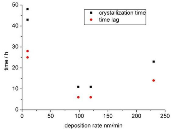
**Figure 3:** Time lag of nucleation and time for complete crystallization of a 500 nm thick a-Si layer on glass for annealing at 600°C as depending on the deposition rate.
