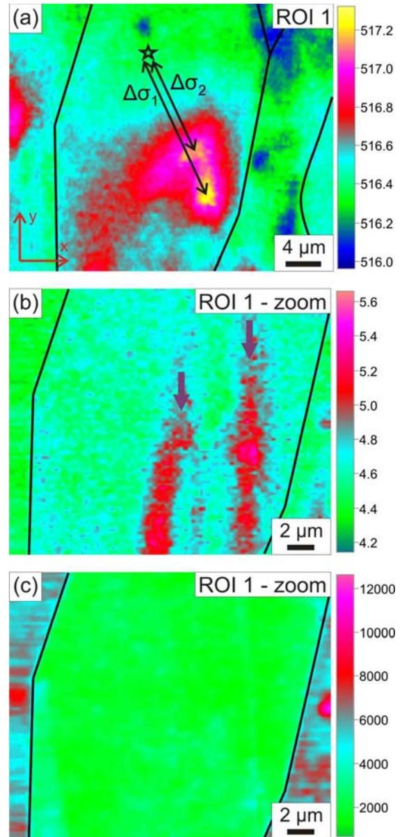
Figure 2: (a) Stress map of ROI 1 equivalent to Raman Si frequency shifts in  $\text{cm}^{-1}$ . The star marks the point where the grain orientation has been determined. Two lateral stress-tensor gradients ( $\Delta\sigma_1$ ,  $\Delta\sigma_2$ ) are indicated with respect to the reference coordinate system. (b, c) Maps of the full width at half maximum (FWHM) in  $\text{cm}^{-1}$  and intensity of the Raman Si peak in counts per second.
