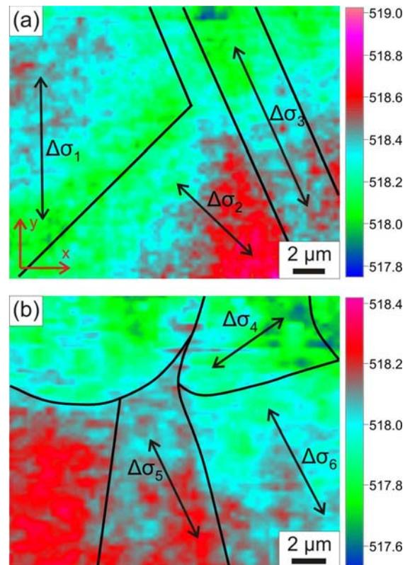
Figure 4: Stress maps of the seed/solid phase epitaxial sample showing inhomogeneous stress distributions at GBs and inside grains. Six lateral average stress gradients ( $\pm 12$  MPa) with respect to the reference coordinate system obtained using Eq. 1 are displayed:  $\Delta\sigma_1=27$ ,  $\Delta\sigma_2=141$ ,  $\Delta\sigma_3=212$ ,  $\Delta\sigma_4=97$ ,  $\Delta\sigma_5=109$ , and  $\Delta\sigma_6=122$  MPa.
